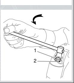
FIG. 7 Pull the hydraulic cartridge (12) from stanchion tube top and make all necessary changes.
