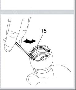
**IMPORTANT:** when removing the oil seal, make sure not to damage slider inner seat. Once removed the oil seals should not be used again. Shiver DG
